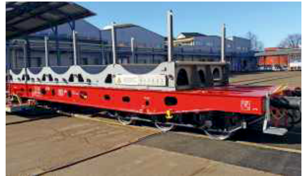
The 'BraCoil' six-axle wagon is intended primarily to carry steel coils but is also designed to handle containers.
