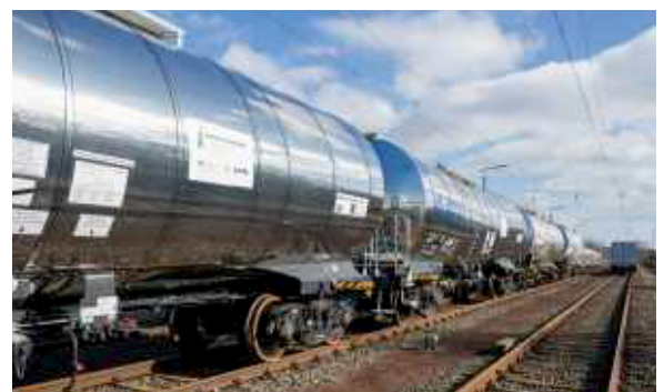
The tank cars are fitted with RC25NT bogies supplied by ELH Eisenbahnlaufwerke Halle.
