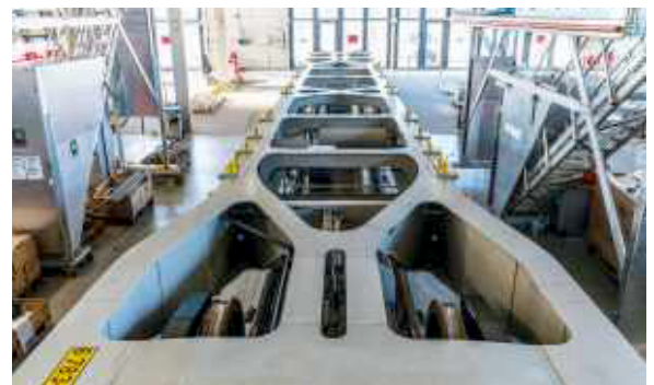
The container wagon features a lightweight skeletal frame and can accommodate combinations of containers of different sizes.
